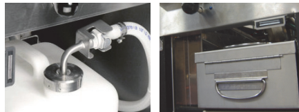
Oil replenished automatically from JIB for multi-well (left) or reservoir for 1-well (right)
